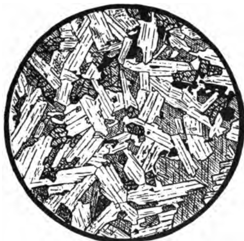
FIG. 32. Diabasic texture, drawn from a microscopic slide of a diabase from Fignon Pt., Minn. The actual field was three eighths inch (1 cm.). The rods of plagioclase are shown enclosing the augite olivine and magnetite. The shaded mineral with light borders is augite; the shaded mineral with heavy borders is olivine. The black mineral is magnetite.
